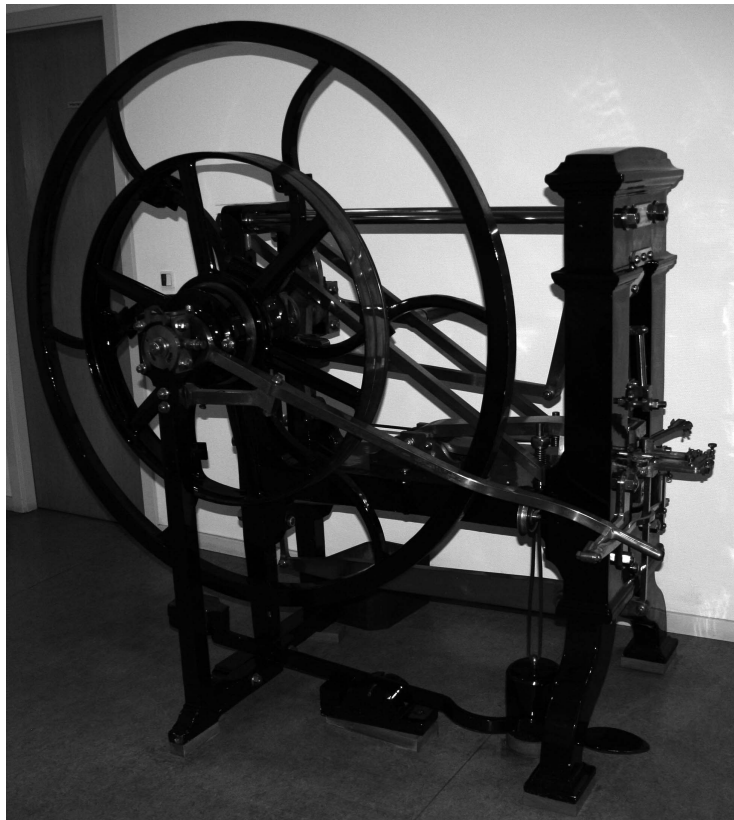
Fig. 5. The second Uhlhorn machine in the realm. It was purchased by the mint in Altona 1842, transported to the mint in Copenhagen 1863 and in use until c. 1950-65, c. 80x200x185 cm.
